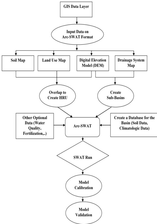
Fig. 3. Diagram for Hydrological Modeling in the SWAT model.
