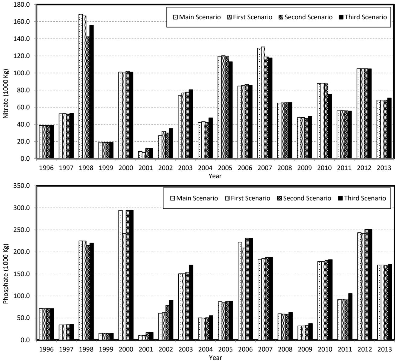
**Fig.7.** (a) Comparison of changes in nitrate leaching from Zanjanrood Basin in irrigation scenarios during the simulation period from 1996 to 2013 and (b) Comparison of changes in phosphate leaching from Zanjanrood Basin in irrigation scenarios during the simulation period from 1996 to 2013.
