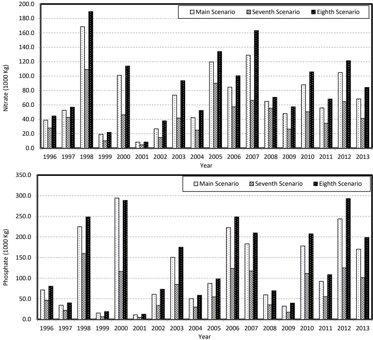
**Fig.9.** (a) Comparison of changes in nitrate leaching from Zanzanrood basin by changing the irrigation method and fertilizer rate, simultaneously and (b) Comparison of changes in phosphate leaching from Zanzanrood basin by changing the irrigation method and fertilizer rate, simultaneously.
