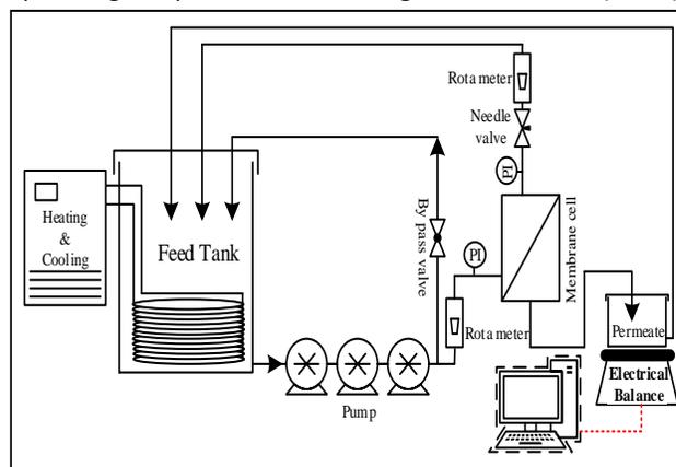
**Fig.1.** Schematic diagram of the bench-scale reverse osmosis system
