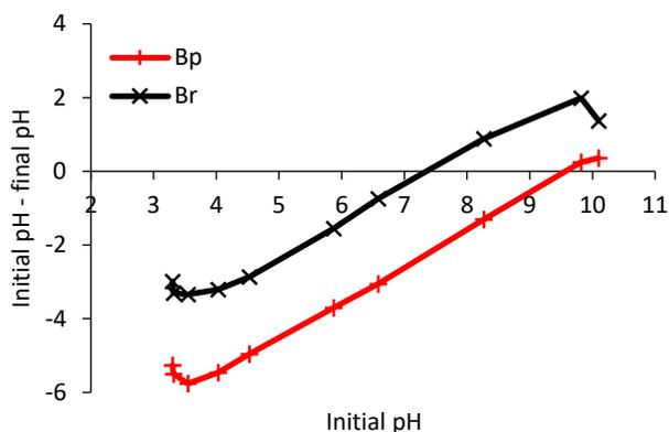
**Fig. 8.** The potentiometric mass titration curves for zero point charge (ZPC) determination of biochars produced from rice husk (Br) and populus wood (Bp). The intersection point of the curve initial pH minus final pH versus initial pH is considered as the amount of point zero charge.
