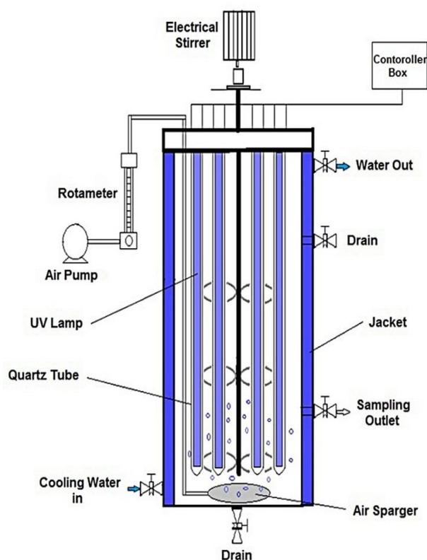
Fig. 2. Schematic diagram of the photocatalytic reactor set up
