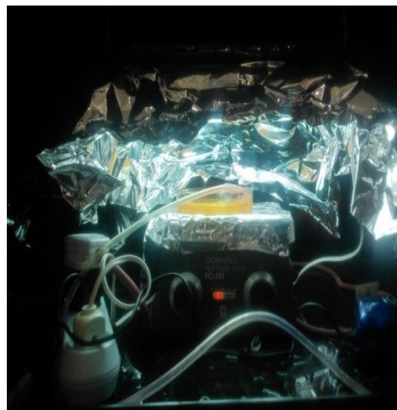
Fig. 13. The inner space of the reactor that shows irradiation on the sample
