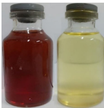
Fig. 7. Transformer oil color before and after reclamation process.
