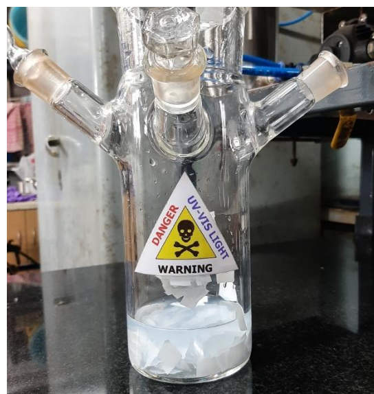
Fig. 22. Photograph of RB 5 Dye (1.3 ppm) degradation using TiO 2 nanofibers- PSF membrane
