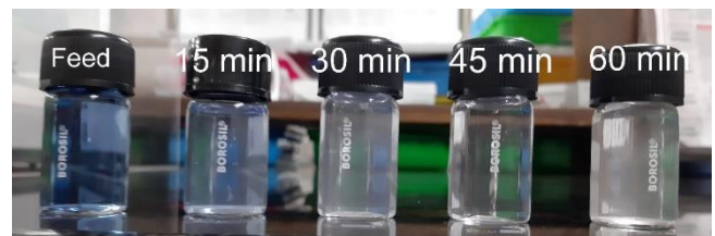
Fig. 12. Photograph of RB 5 Dye feed and samples collected at different time intervals in \text{TiO}_2 photocatalysis.
