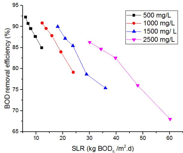
**Fig. 10.** Calculated BOD removal efficiency versus surface loading rate.
