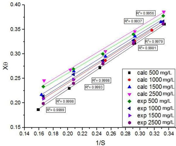
Fig. 6. Performance evaluation of MBSBR using the Optaken and Grau Second Order Substrate Removal Model.
