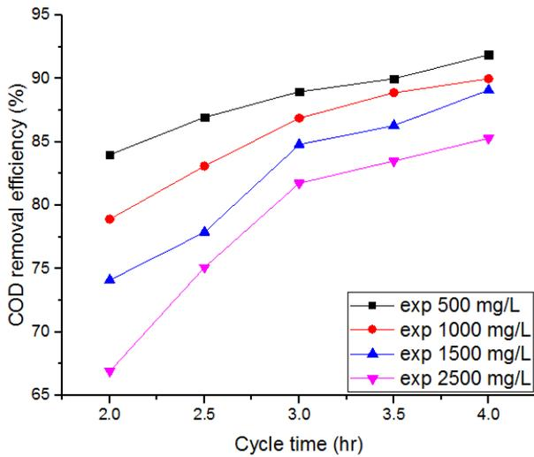
Fig. 11. Experimental COD removal efficiency versus cycle time.
