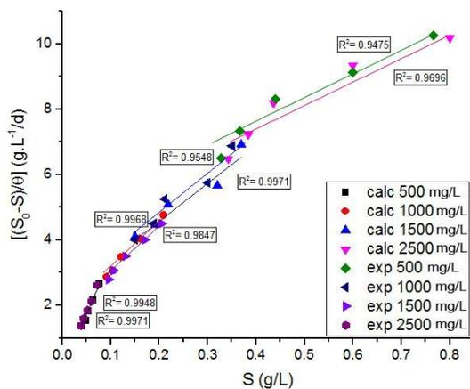
**Fig. 5.** Performance evaluation of MBSBR using First Order Kinetic Removal model.
