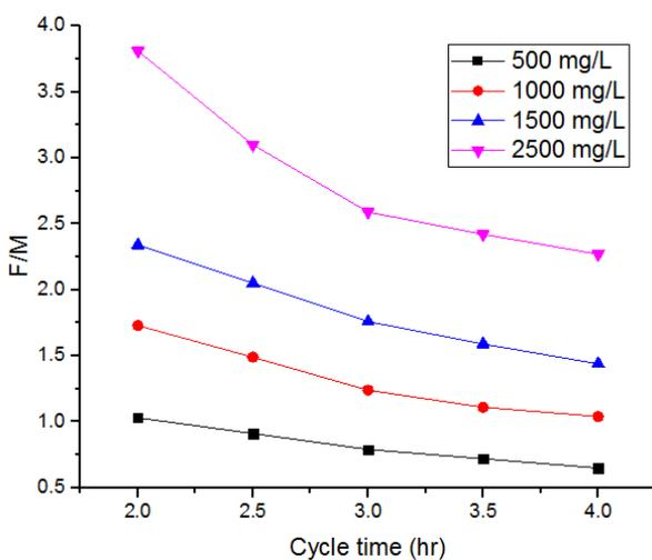
Fig. 12. Experimental F/M ratio versus cycle time.
