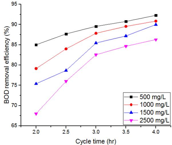
Fig. 7. Calculated BOD removal efficiency versus cycle time.
