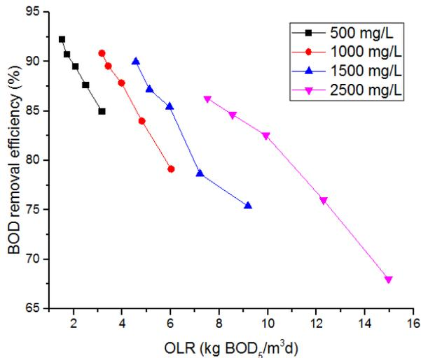
**Fig. 9.** Calculated BOD removal efficiency versus Organic loading rate.
