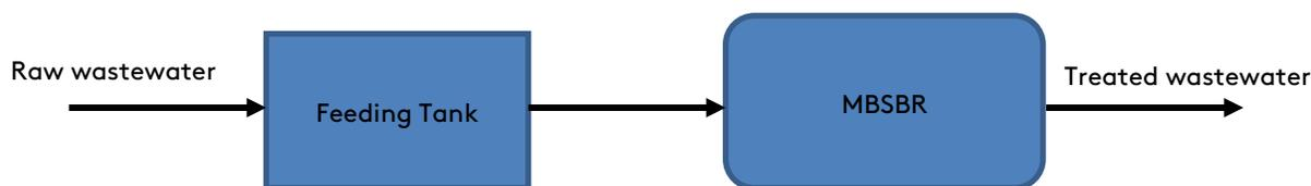
**Fig. 1.** Modelled MBSBR system.
