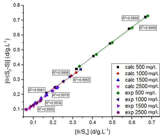
**Fig. 4.** Performance evaluation of MBSBR using Modified Stover Kincannon model.
