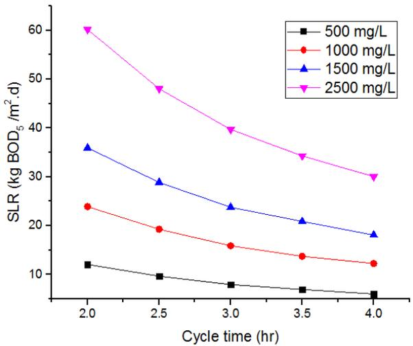
Fig. 8. Experimental surface loading rate versus cycle time.
