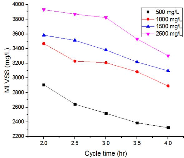
Fig. 13. Experimental MLVSS concentration versus cycle time.
