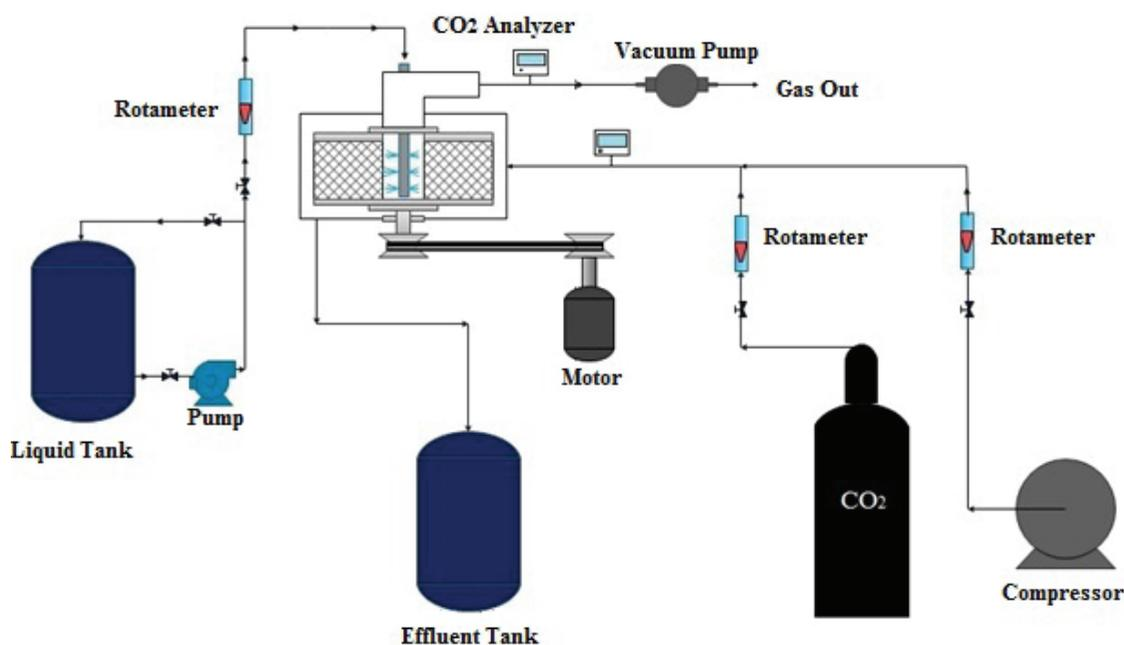
**Fig. 1.** Rotating packed bed diagram.
