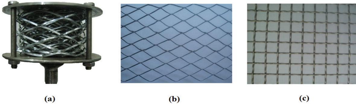
Fig. 2. (a) Rotor. (b) Expamet Packing. (c) Wire Mesh Packing.
