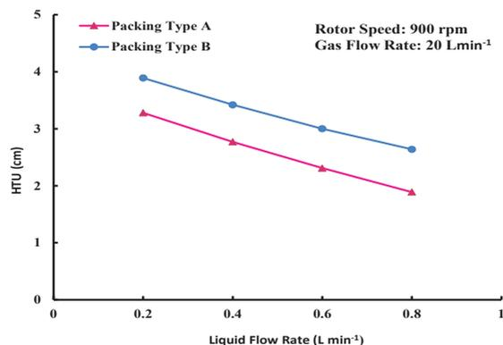
Fig. 6. Dependence of HTU on liquid flow rate for different packing types and 30 wt% MEA.
