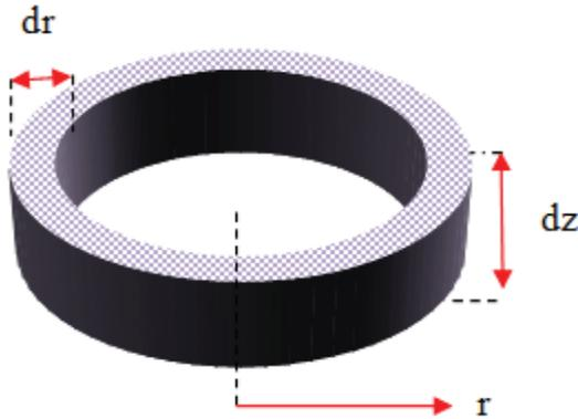
Fig. 3. Differential volume of rotating packed bed.
