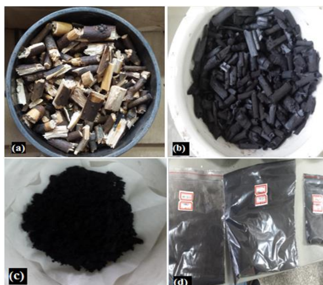
Fig. 1. Biochar preparation: (a) Before pyrolysis, (b) after pyrolysis, (c) biochar powder after grinding and sieving and (d) biochar powder packed to store in a desiccator for future use.
