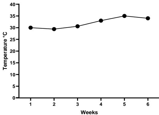
Fig. 6. Variation of the temperature in the batch sequential reactor.
