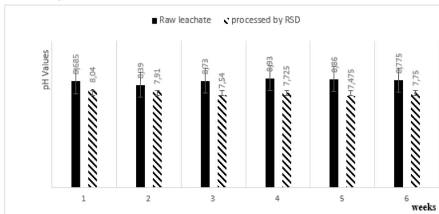
Fig. 4. Variation of the pH in the sequential batch reactor.
