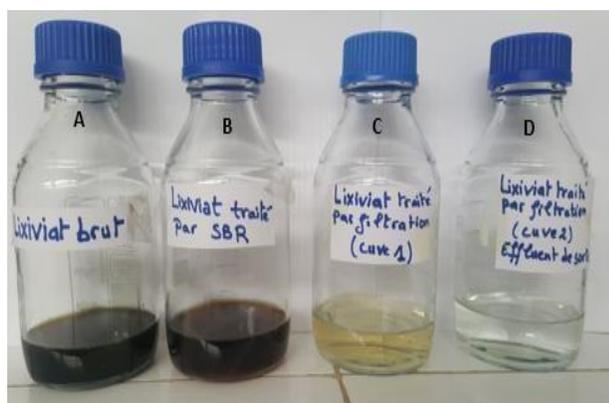
**Fig 9.** Discoloration of leachate treated with SBR and filtration A: Raw leachate, B: leachate treated by SBR, C&D: leachate treated by filtration after coupling (tank 1 and tank 2).
