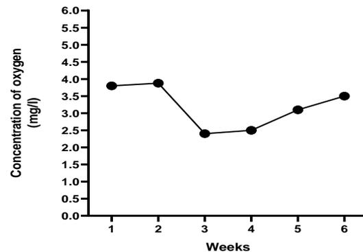
Fig. 5. Variation of dissolved oxygen in the sequential batch reactor.
