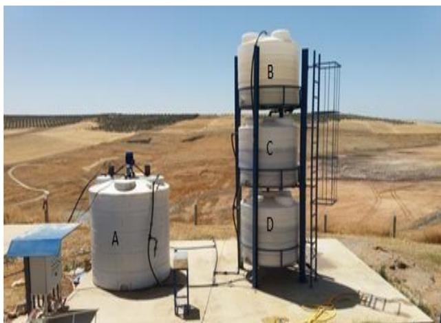
**Fig. 2.** The pilot at the Fez landfill, A= The Sequential Batch Reactor (SBR), B= Column of storage, C&D= Columns of filtration.
