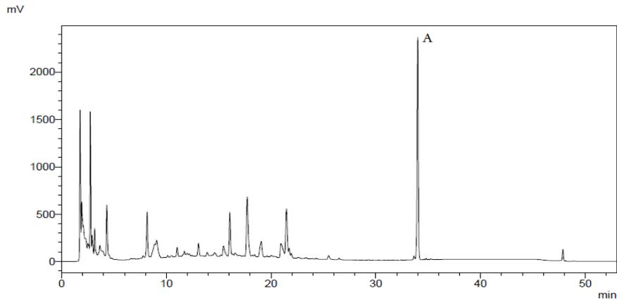
Fig. 3. Chromatogram of leachate with detergent peak at t = 35 min A = Triton.
