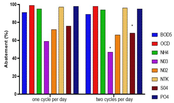
Fig. 7. Rate of reduction of the parameters after treatment of the leachate by the SBR with one and two cycles per day.
