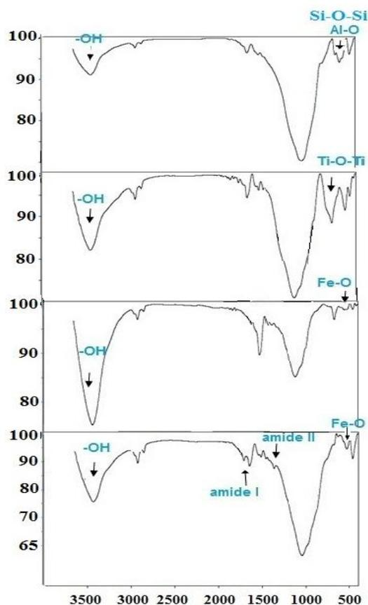
Fig. 2. FT-IR spectrum of Kissiris, Kissiris/TiO<sub>2</sub>, Kissiris/TiO<sub>2</sub>/Fe<sub>3</sub>O<sub>4</sub>, and Kissiris/TiO<sub>2</sub>/Fe<sub>3</sub>O<sub>4</sub>/GOx.
