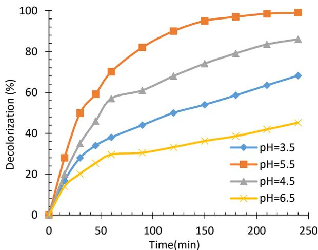
**Fig. 6.** Effect of pH value on pseudo-first order rate constant during heterogeneous bio-Fenton oxidation treatment;  $[MG]_0 = 20 \text{ mg/L}$ ,  $[glucose]_0 = 20 \text{ mM}$ , 1 g Kissiris/ $Fe_3O_4/TiO_2/GOx$ ,  $T = 35^\circ \text{C}$ .
