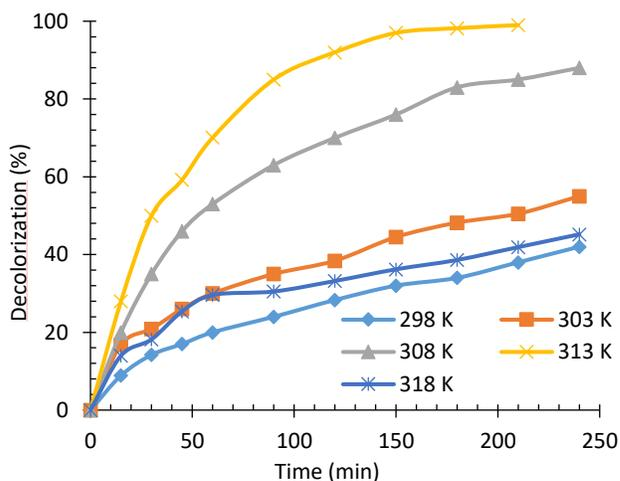
**Fig. 7.** Effect of temperature on pseudo-first order rate constant during heterogeneous bio-Fenton oxidation treatment;  $[MG]_0 = 20 \text{ mg/L}$ ,  $[glucose]_0 = 20 \text{ mM}$ , 1 g Kissiris/ $Fe_3O_4/TiO_2/GOx$ ,  $\text{pH} = 5.5$ .
