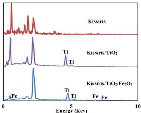
Fig. 1. EDX spectrum of Kissiris, Kissiris/TiO<sub>2</sub> and Kissiris/TiO<sub>2</sub>/Fe<sub>3</sub>O<sub>4</sub>
