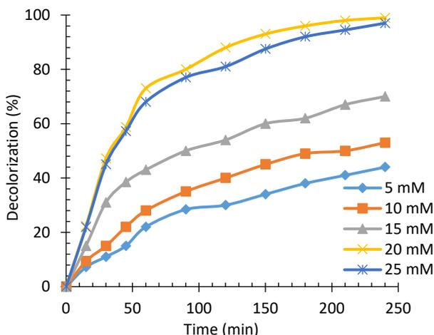
**Fig. 5.** Effect of initial glucose concentration on pseudo-first order rate constant during heterogeneous bio-Fenton oxidation treatment;  $[MG]_0 = 20 \text{ mg/L}$ , 1 g Kissiris/ $Fe_3O_4/TiO_2/GOx$ ,  $T = 35^\circ \text{C}$ .
