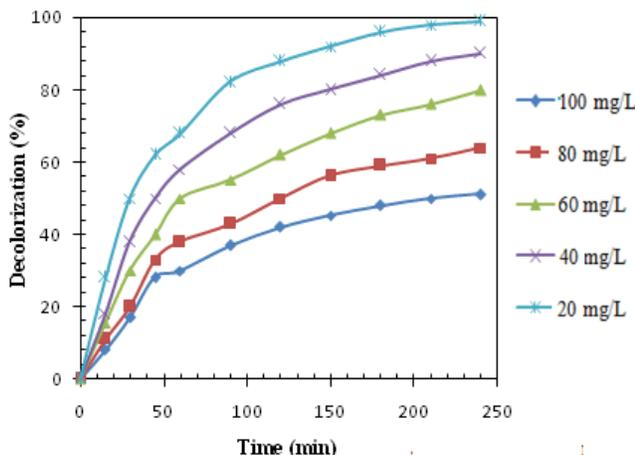
Fig. 4. Effect of initial concentration of dye on pseudo-first order rate constant during heterogeneous bio-Fenton oxidation treatment; [glucose]<sub>0</sub>=20 mM, 1 g Kissiris/Fe<sub>3</sub>O<sub>4</sub>/TiO<sub>2</sub>/GOx, T= 35°C.
