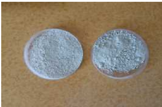
Fig. 2. Surfactant-modified Sabzevar nanozeolite
