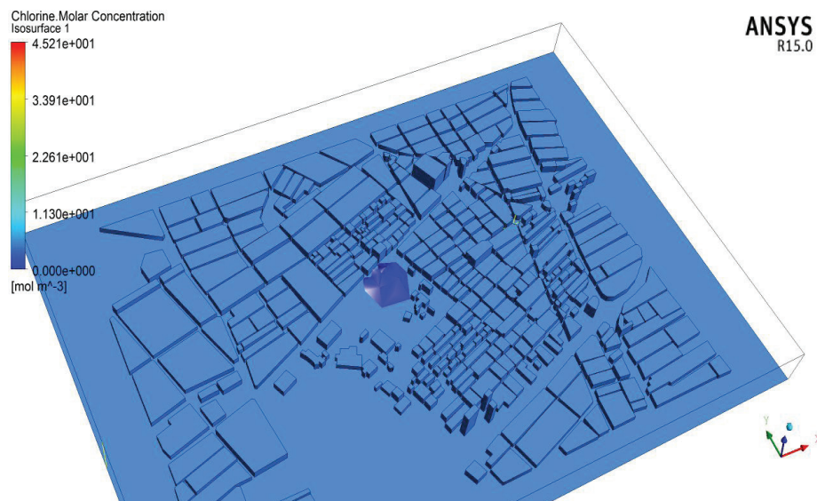
Fig. 10. Chlorine gas cloud of 10 \text{ mg L}^{-1} after 1000 seconds (dark blue polygon in the middle).
